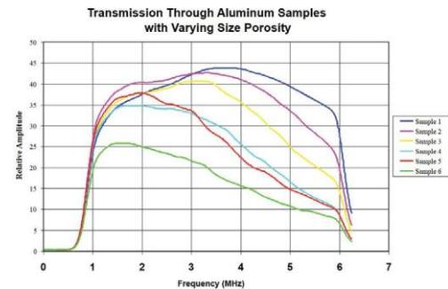
As frequency increases, or wavelength decreases, the amplitude of the ultrasonic signal decreases. The defect can be estimated by the roll-off energy in the spectrum.
