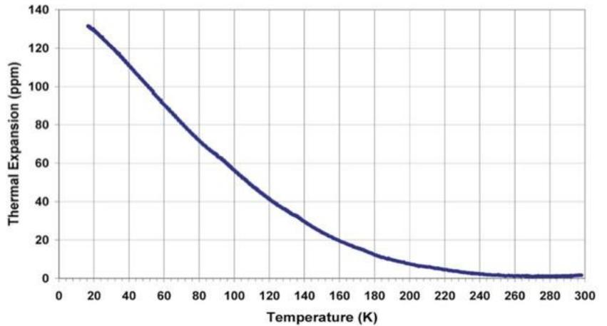
Kratos SRE has developed unique facilities for measuring thermal expansion with ultra-high accuracy from >350 K down to below 30 K. Using interferometers and a proprietary optical flagging system, CTE accuracy of better than 20 parts-per-billion is standard. Sample sizes can range from 1 cm to 1 meter in length.
