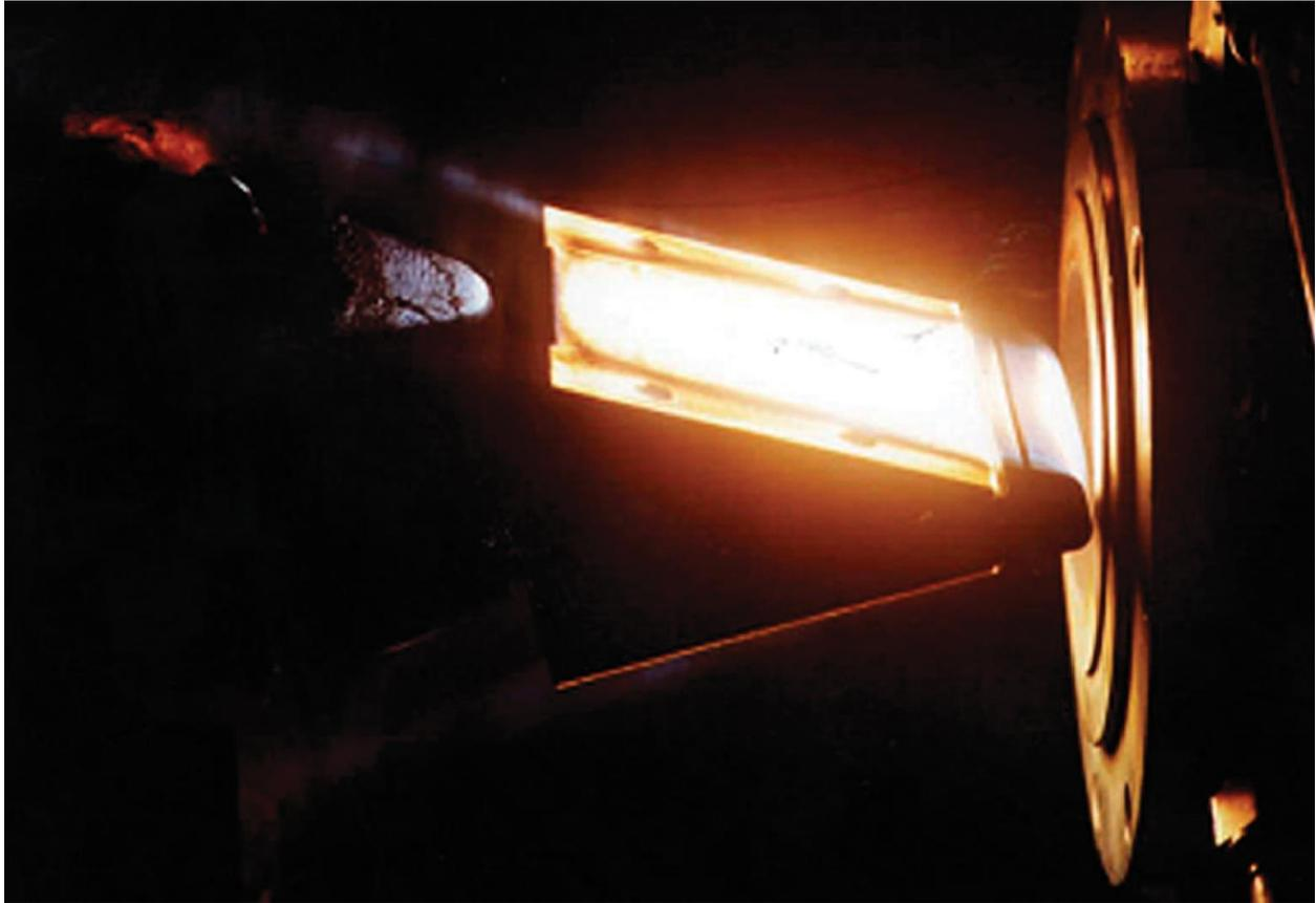
Since 1995, Kratos SRE has led hundreds of ground tests at various test facilities around the U.S. Conducting ground tests and performing post-test analysis on thermal protection materials designed for hypersonics applications, remains a key area of expertise for the Hypersonic Structures Department. The ground tests are carried out in either commercial or government supported test facilities using hardware and instrumentation developed and fabricated by Kratos SRE.
