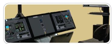
Realistic cockpit interactions enable immersive avionics System simulation. MBRAT provides student training through simulation of both cockpits on multiple touch- screen monitors.
