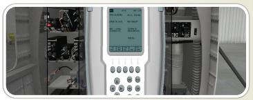
Virtual test set to troubleshoot and diagnose faults. Modeled after tactical test set, MBRAT enables students and instructors to perform Remove and Replace Tasks, component troubleshooting, along with the use of simulated virtual aircraft test sets.
