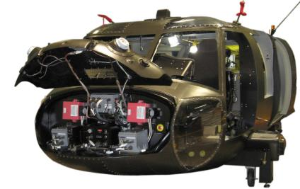
The BHAT-M supports all the critical tasks necessary to train MOS (Military Occupational Specialty) 15N10/30 Avionics Mechanics. Typical 15N training tasks include trouble shooting, isolation of faults and restoration of functionality.
