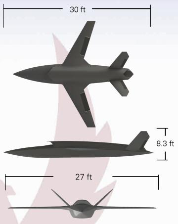
Length30 ftWingspan27 ftDry Weight2,500 lb
