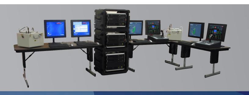
The Unmanned Vehicle Control System is a field proven C2 system based on the MONTAGE architecture used to control remotely piloted vehicles or target drones. The system can control multiple full and/or sub-scale fixed and rotary wing aerial targets and sea surface targets to a range of 200 nm line of site, or up to 330 nm with a minimum of 12dB of margin if using the optional relay system, using differentially corrected GPS position data.
