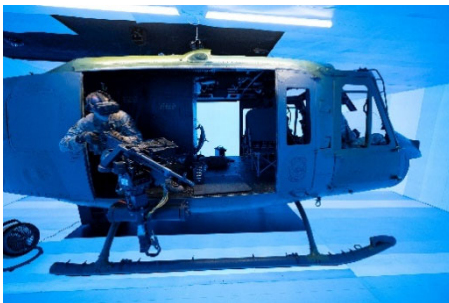
Kratos' UH-1 Multi-Position Aircrew Virtual Environment Trainer (MP-AVET) enclosed in a Kratos mixed reality holodeck
