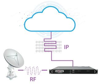
OpenSpace SpectralNet digitizes the RF into IP for transport and signal processing using OpenSpace quantum products or the OpenSpace Platform.
