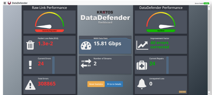
OWTP optimizes data transfer rates, controls latency, insures data delivery and provides network situational awareness.
