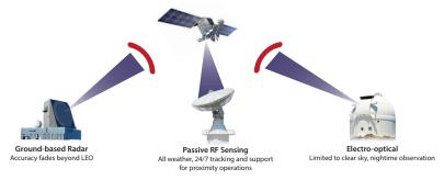
The two main sensor types for SDA data: Radar and Electro-Optical (EO). Each offers strengths, but also limitations. RF data can fill the gaps to enhance SDA.
