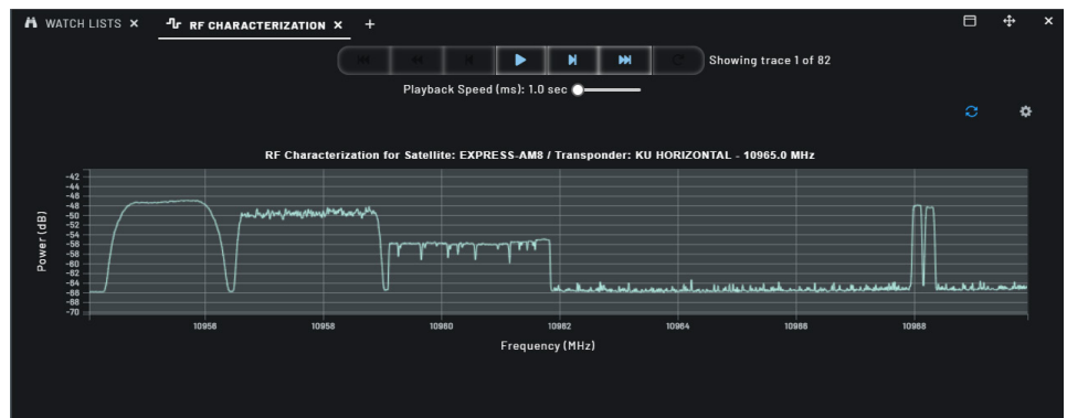
RF data is collected and analyzed over a period of time. This chart indicates activity following a satellite anomaly affecting the services of a global satellite operator.
