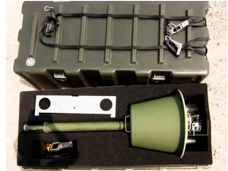
Photo representing a dual optic feed system
