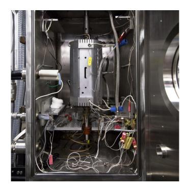
Kratos SRE's Variable Atmosphere Temperature and Pressure (VATP) Facility was built for evaluation of hypersonic vehicle leading-edge materials via mission performance tests in realistic service environments, such as variable temperature, atmosphere, pressure, and load.
