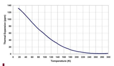
Kratos SRE has developed unique facilities for measuring thermal expansion with ultra-high accuracy from >350 K down to below 30 K. Using interferometers and a proprietary optical flagging system, CTE accuracy of better than 20 parts-per-billion is standard. Sample sizes can range from I cm to I meter in length.
