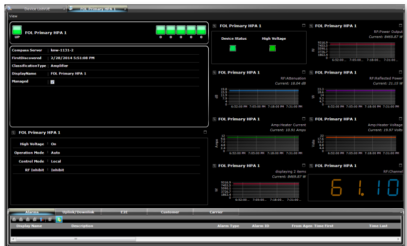
▲ A drill down view from NeuralStar SQM shows the status of a device in the downlink service.
