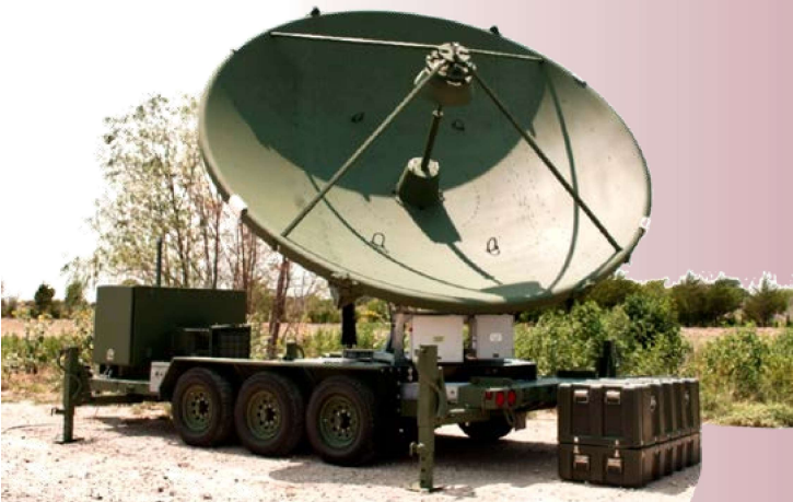
Trifold transportable antenna system. Photo provided by Kratos.
