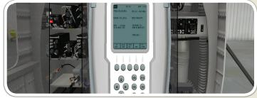
Provides virtual test set to troubleshoot and diagnose faults. Modeled after tactical test set. The MBRAT enables students and instructors to perform Remove and Replace Tasks, component troubleshooting, along with the use of simulated virtual aircraft test sets.
