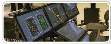
Realistic cockpit interactions enable immersive avionics system simulation. MBRAT provides student training through simulation of the CH-47F cockpit on multiple touch screen monitors.
