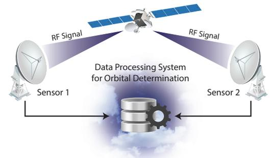
*Kratos measures satellite signals from multiple sensors to determine where a satellite is in orbit and to detect when it is maneuvering.*
