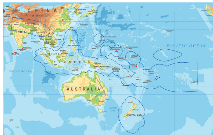
Kacific's network consists of 56 spot beams servicing 25 countries across Asia Pacific. Source: Kacific Broadband Satellites Group
