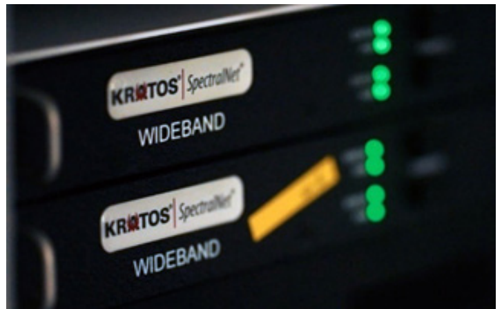
SpectralNet Wideband digitizers at Kacific gateways convert RF signals into IP packets to remove distance barriers in RF signal transport. Source: Kratos
