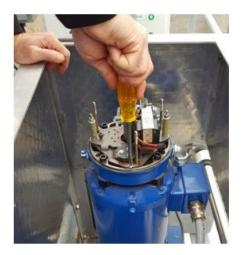
Figure 4-14: Reinstalling Support Plate
