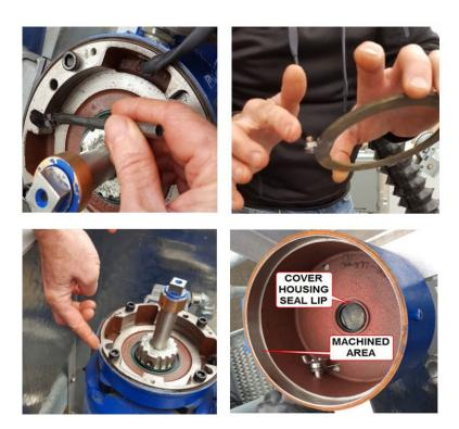
Figure 4-12: Applying Silicone Grease
