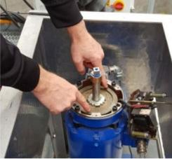
Figure 4-13: Reinstalling Disc Pack
