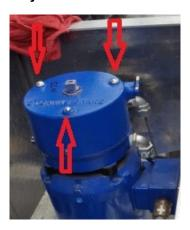
Figure 4-7: Cap-Nuts on Top of Brake Assembly
