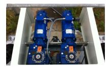
Figure 4-5: Azimuth Brakes
