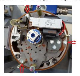
Figure 4-8: Support Plate Screws
