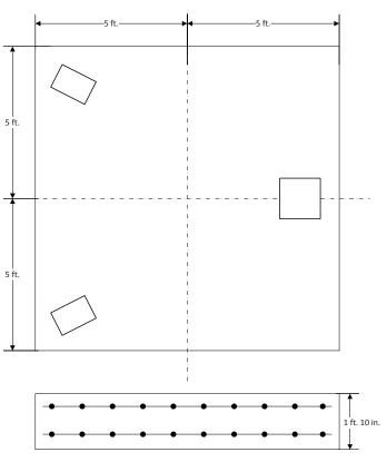
pads (based on 15 ton crane) 8ft (2.4m) minimum Assembly area for mount and antenna Azm = Azimuthdirection of mount 15ft (4.5m) minimum 5ft (1.5m) minimum 8ft (2.4m) minimum 25ft (7.5m) 30ft (9m) minimum clearance on either side of foundation for crane access
