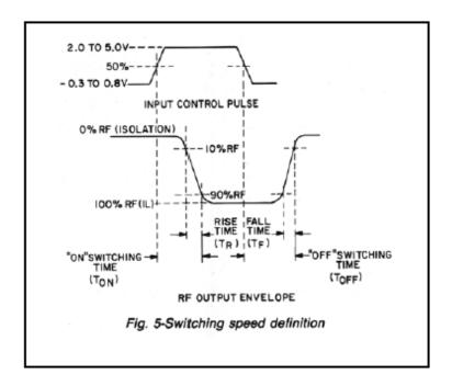
**ON TIME** is measured from the 50% level of the input control signal to the 90% point of the square-law detected RF power, when the unit is switched from full OFF to full ON.
