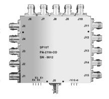
The common port of standard absorptive multi-throw switches will be reflective, only when all ports are turned OFF. If there is a need for this port to remain matched under these conditions, it can be realized either by employing an additional port, to which an external termination is connected, or by providing automatic connection of an internal termination to the common port in a custom design.
